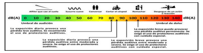
The diagram above shows the tolerable range without impairment and the impact on the ear of different sound levels and exposure times. Look at the technical data sheet of a hearing aid and, based on this information, answer the question.
